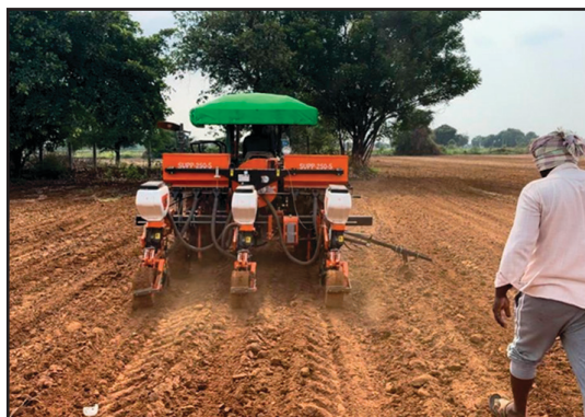
Monitoring Sowing of HDPS Cotton Using a Pneumatic Planter
