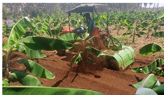
Demonstration of inter-cultivator cum ridger for banana - KVK Erode (TN)
